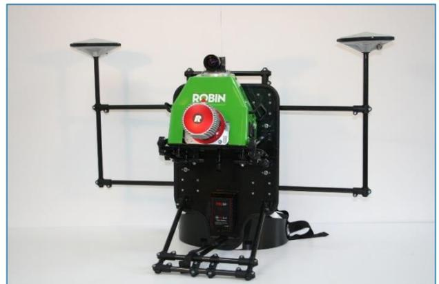
FIGURE 9: SYSTÈME LIDAR PÉDESTRE 3D LASER MAPPING ROBIN
