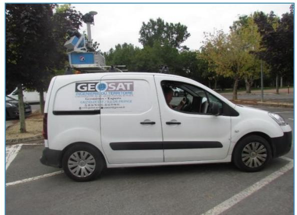
FIGURE 8: VOITURE EQUIPEE DE LA TECHNOLOGIE LIDAR
