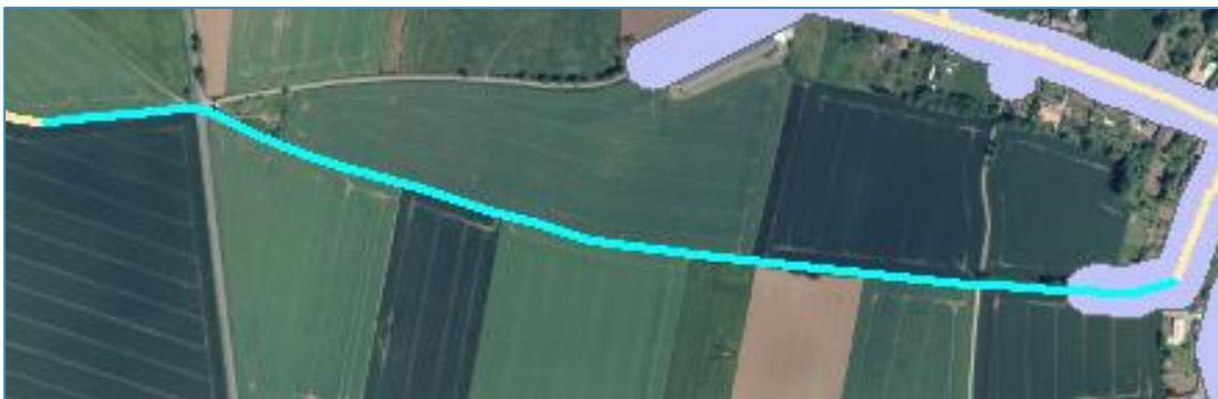
**FIGURE 25: PROBLEME : LA SECTION DU RESEAU D'EAU SELECTIONNEE COMPORTE UNE ENORME PARTIE HORS DU TAMPON MAIS TOUTE SA LONGUEUR SERA PRISE EN COMPTE POUR LE CALCUL**
