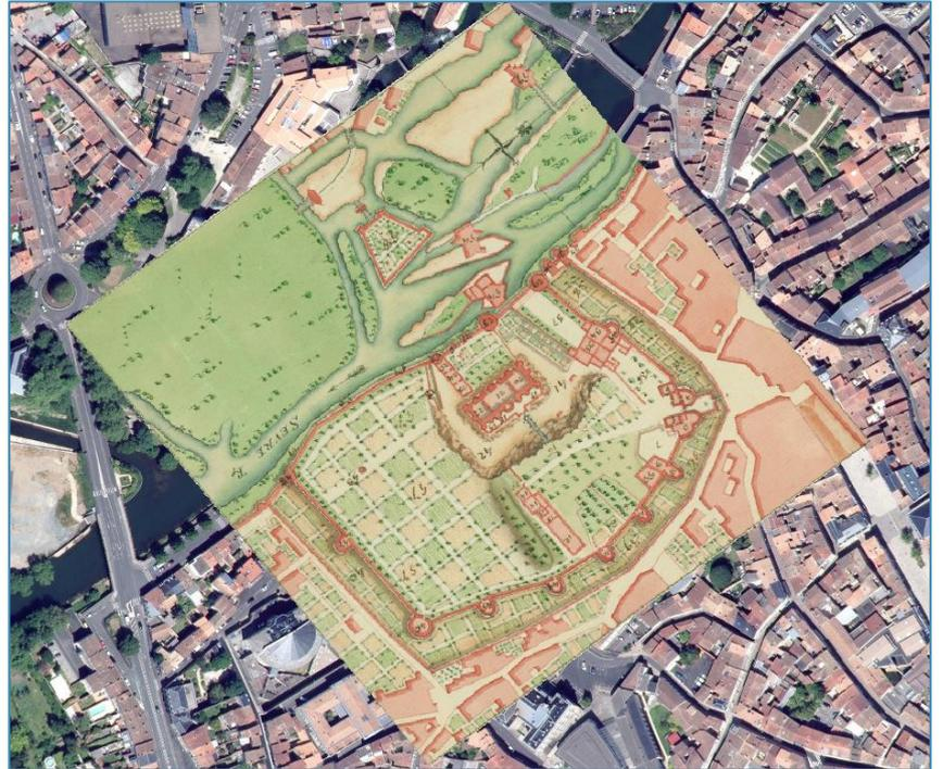
**FIGURE 81: GEOREFERENCEMENT DU PLAN SUR L'ORTHO**
