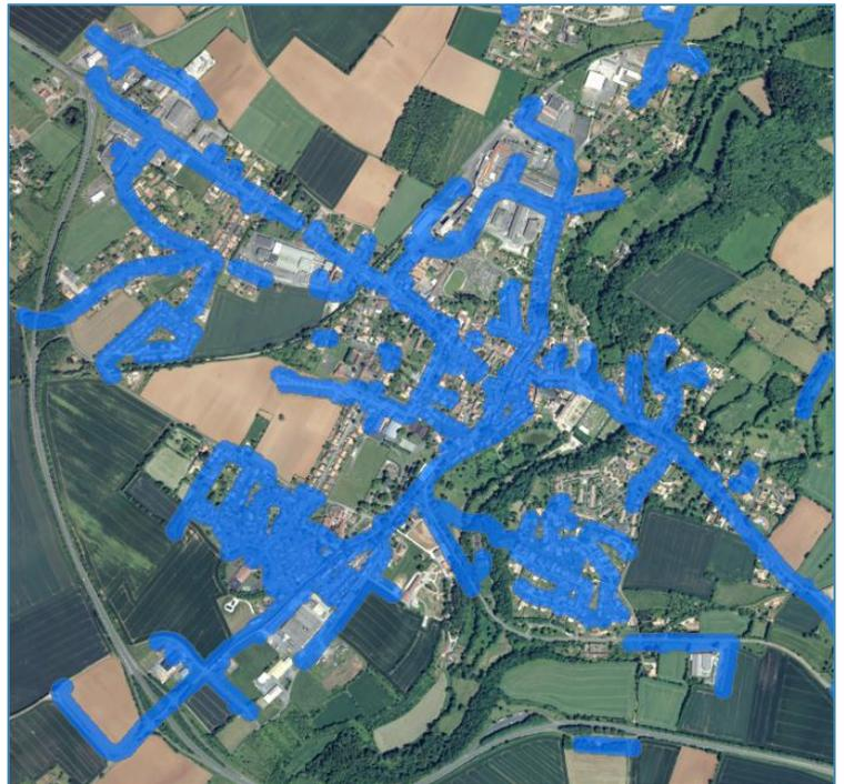
**FIGURE 26: TAMPON DE 25M AU NIVEAU DU RESEAU ELECTRIQUE SOUTERRAIN A CELLES-SUR-BELLE**
